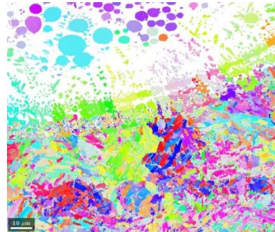
(b) Inverse pole figure of steel in the mixing zone, red: \langle 001 \rangle , green: \langle 101 \rangle , blue: \langle 111 \rangle .
