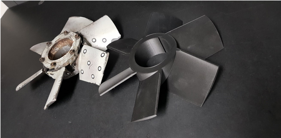
Figure 2: Fan for a motor and replacement part, made in the field by Fieldmade for Equinor during Trident Juncture 18. Since the original fan had gone out of production, reverse engineering and reproduction of this part was the only alternative to replacing the entire motor unit. Courtesy of Fieldmade and Equinor.
