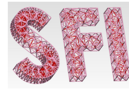
Figure 4. Example of so called lattice structures (truss work) that can be built by AM.
