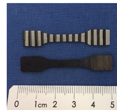
Figure 18. Tensile test samples of elastomers produced by additive manufacturing. Top: A multimaterial test specimen produced by combining two different elastomers during one additive manufacturing technique. Bottom: A single material elastomer test specimens.
