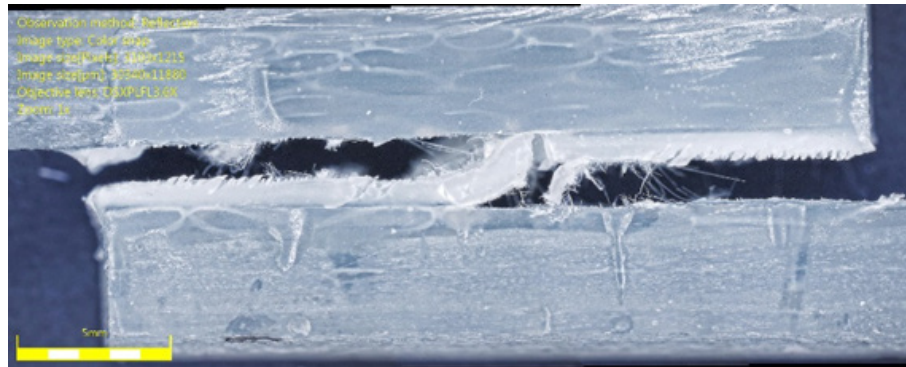
Figure 2. Adhesive bond strength in bonding composite laminates is tested in a single lap shear test.
