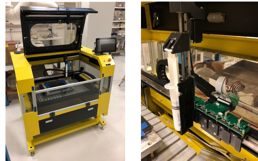
Figure 9. A: The Hydra additive manufacturing R&D platform (shown here with a white extrusion deposition module). B: Close-up of the 5 head module positions, one of which is loaded with a simple syringe dispensing head module.
