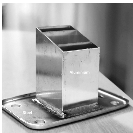
Figure 3. Aluminium crash box was joined to a steel back plate using the CMT process in the IPN Optimals project. Two aluminium-steel components were welded to an aluminium bumper beam to form a crash management system.
