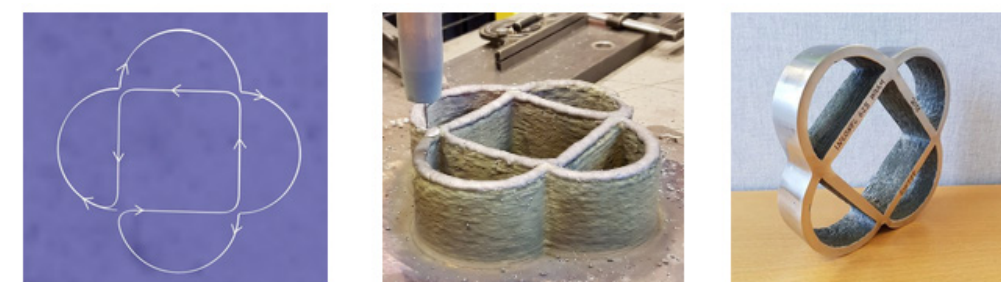
Figure 2. Here we can see the path for the weld in order to avoid actual crossings within each layer, and the final metal structure before and after processing. The dimensions are approximately 16 x 16 cm 2 .
