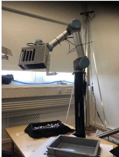
Figure 4. The physical setup consists of a UR5 robot with a Zivid 3D camera and vacuum gripper.
