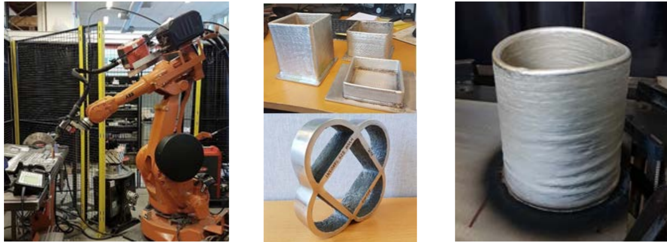
Figure 5a. Robot cell at SINTEF Industry with ABB robot manipulator and Fronius welding equipment. Figure 5b. Box structures and «Chinese knot» built with fixed orientation of welding gun, mapping challenges related to corners and intersections. Figure 5c. Cup structure built using set-based control to allow for 6° slack in orientation of welding gun.
